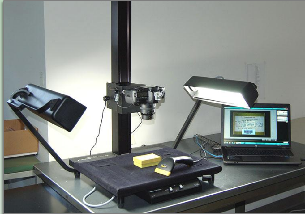
Example: imaging workstation with Bencher Copymate II copystand, lights included
